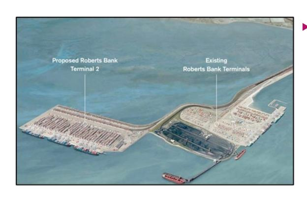
Port of Vancouver intends to expand the existing Roberts Bank Terminal in an effort to increase container handling capacity. A whole new terminal is planned to be created, which will add 2.4 million TEUs (20ft equivalent unit containers) of container capacity to meet the anticipated growth in demand for container capacity to 2030. Seabird Island is being consulted on this project to due to the environmental impact it may have on the Salish Sea.
